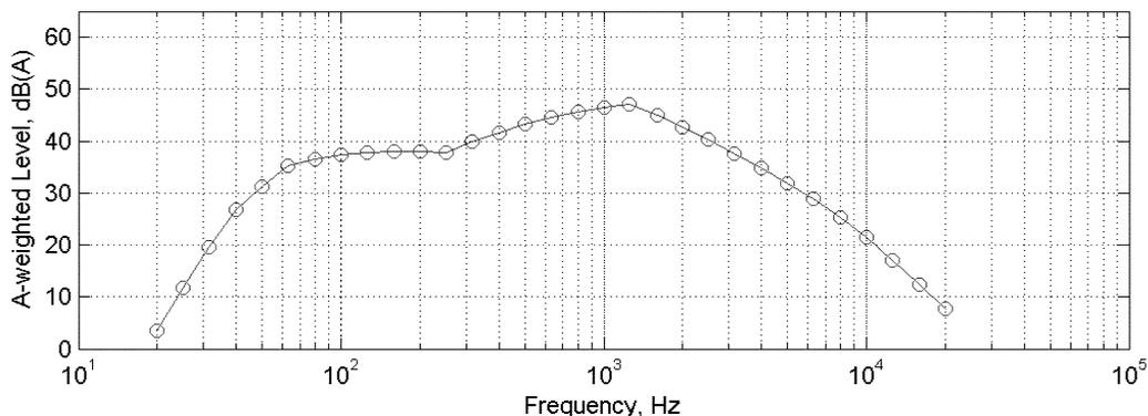
**Figure 2. A-weighted Spectrum and Ambient at 55 A-weighted dB**
