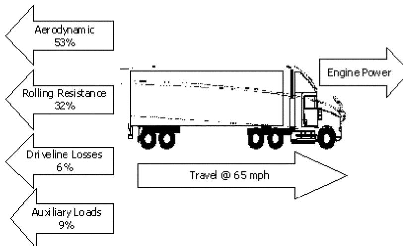
Figure I-1: Combination Tractor and Trailer Loads<sup>24</sup>
