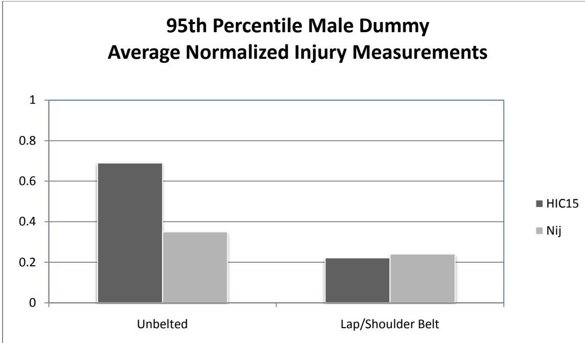
**Figure IV-18: 95<sup>th</sup> Dummy Restraint Comparison – Average Normalized Injury Measurements**
