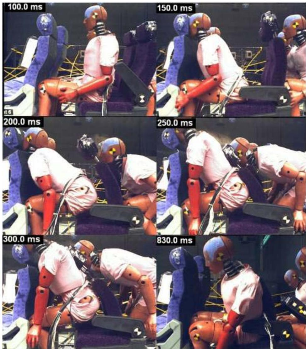
Figure IV-9: Unbelted Sled Test – 50<sup>th</sup> Percentile Male Dummy
