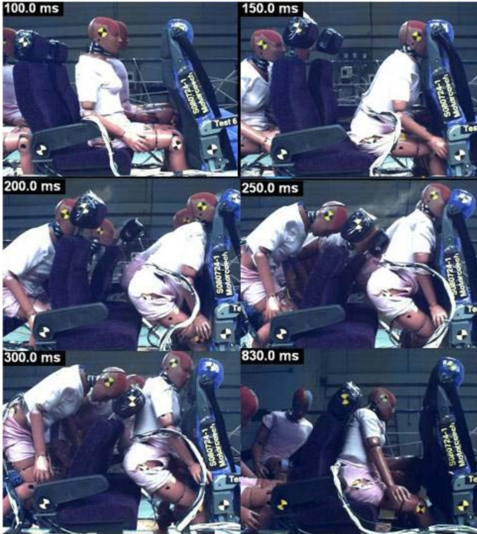
**Figure IV-10: Unbelted Sled Test – 5<sup>th</sup> Percentile Female Dummy**
