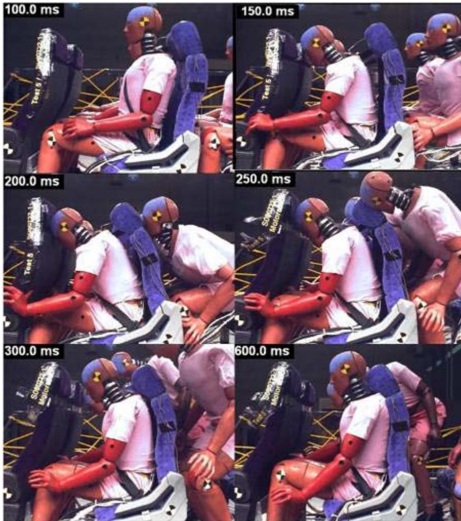
**Figure IV-15: Lap/Shoulder Belted Sled Test – 50<sup>th</sup> Percentile Male Dummy (Rear Loading)**
