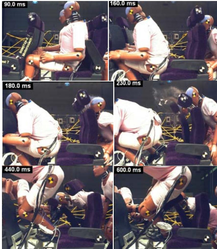
**Figure IV-8: Unbelted Sled Test – 95<sup>th</sup> Percentile Male Dummy**
