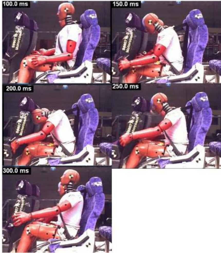
**Figure IV-14: Lap/Shoulder Belted Sled Test – 50<sup>th</sup> Percentile Male Dummy**
