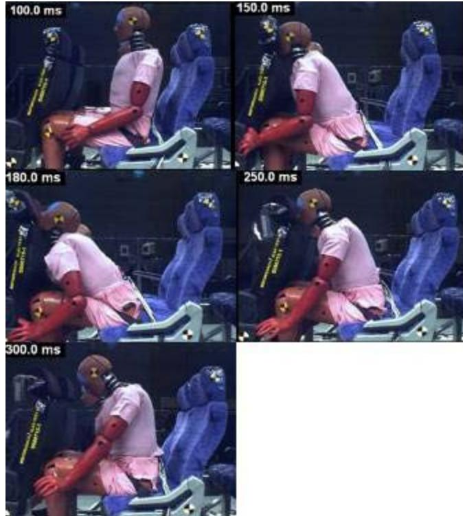
**Figure IV-12: Lap Belted Sled Test – 50<sup>th</sup> Percentile Male Dummy**
