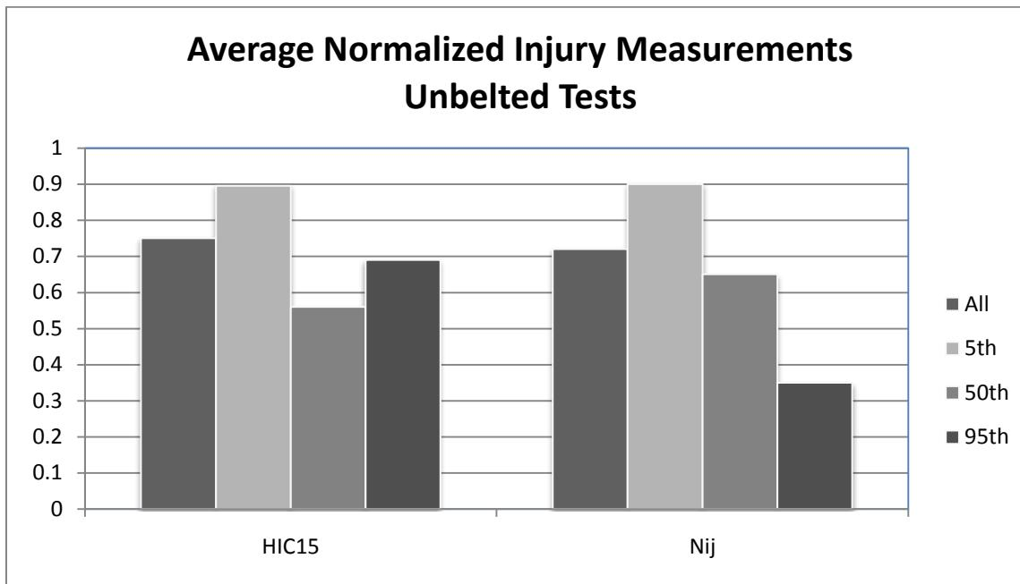
**Figure IV-11: Unbelted Tests – Average Normalized Injury Measurements**
