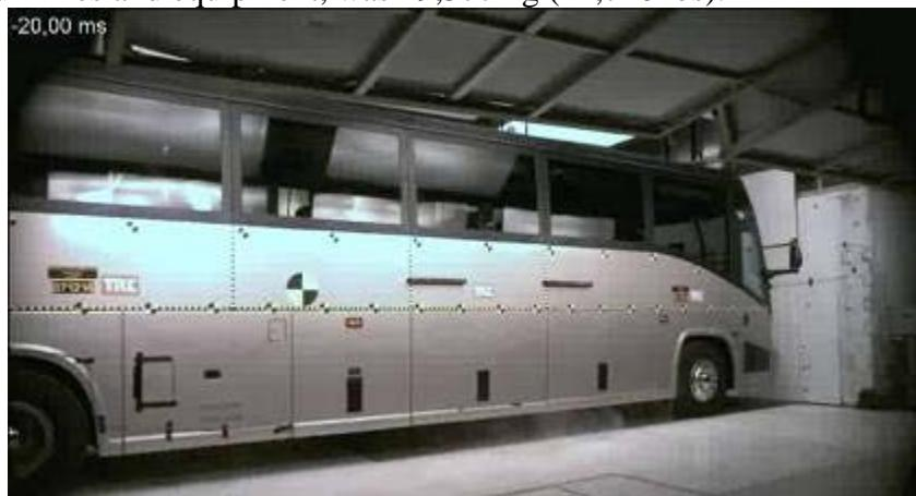
**Figure IV-1: Pre-test Photo of Full-Scale Rigid Barrier Crash Test**
