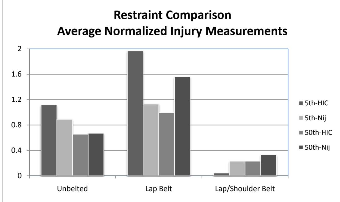
**Figure IV-17: Restraint Comparison – Average Normalized Injury Measurements**
