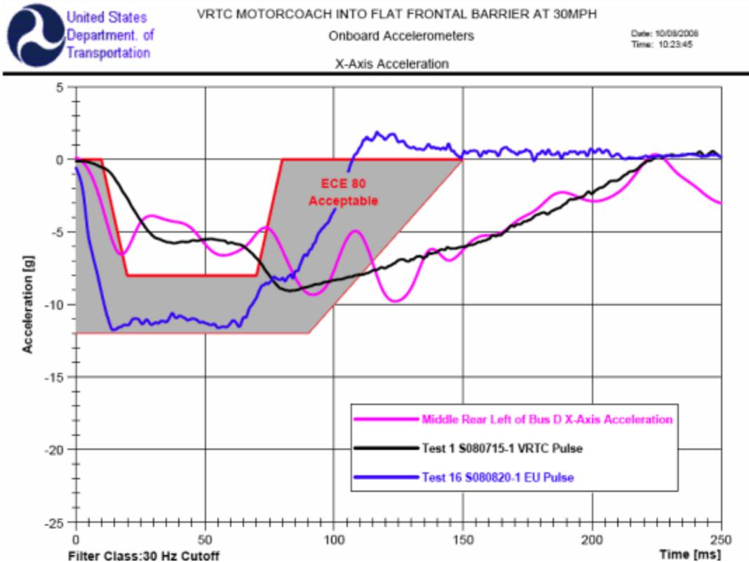
**Figure IV-7 Crash Test and Sled Test Pulses**
