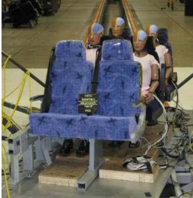
**Figure IV-6: 15-Degree Offset Sled Test Configuration Set-up**
